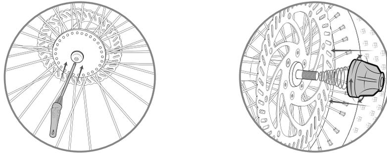
**Step 3:** Insert front tire into front fenders. Once mounted, simply tighten the black bolt and move the release latch to the upward position to close.
