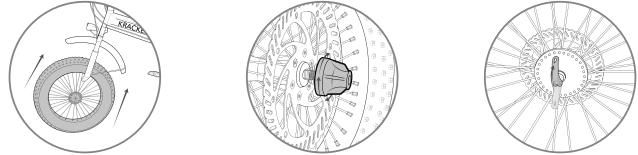
**Pro Tip:** Check the tension by moving your quick release to the up position every couple of turns of the bolt. Release latch should leave a small indention in your hand. If to tight simply unscrew the bolt till you can fasten the latch. Should be snug.
