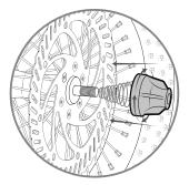
Step 3: Insert front tire into front fenders. Once mounted, simply tighten the black bolt and move the release latch to the upward position to close.
