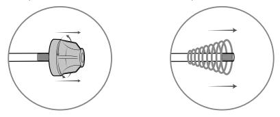
**Step 2:** Unscrew the black bolt and remove only 1 spring. Insert the skewer into the front rim ( the release latch should be on opposite side of the break rotor. ) Once inserted, place back the spring ( large side of spring facing out ) and give the black bolt a couple of turns just so it's able to not fall off. Do not tighten yet. Leave a gap.
